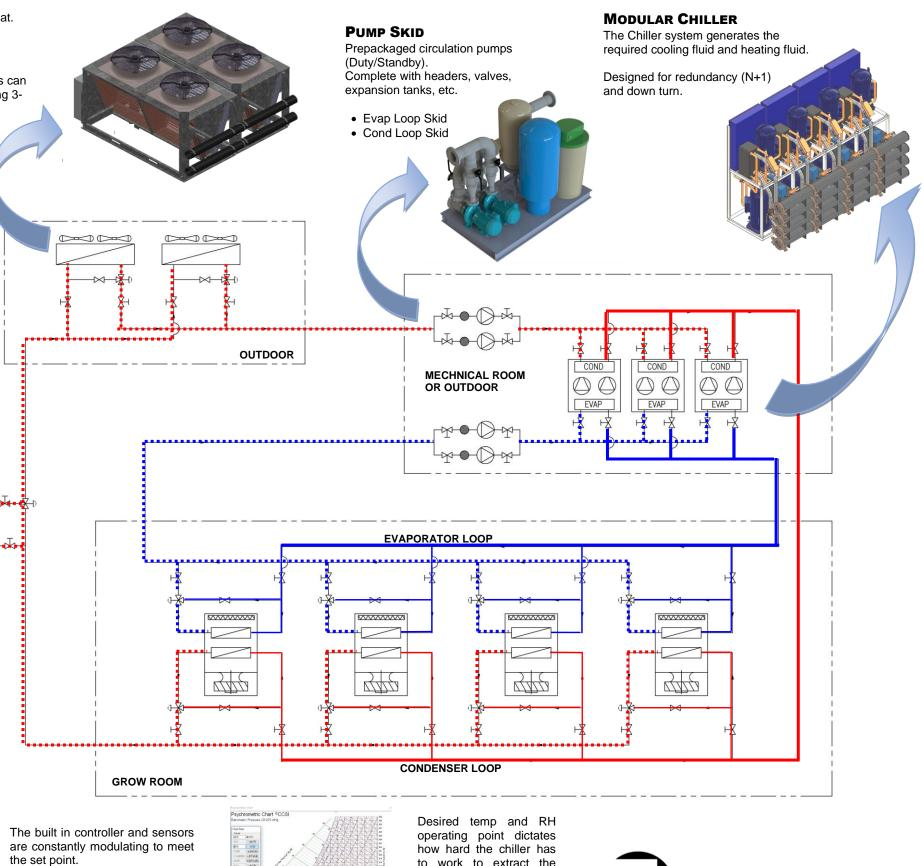
The controller communicates directly with the main control system allowing for changing set points following the grower's recipe.
